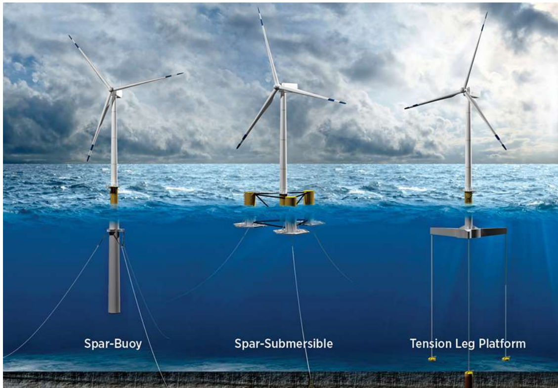
Figura 1. Offshore wind floating foundation concepts (Fonte: IRENA)
